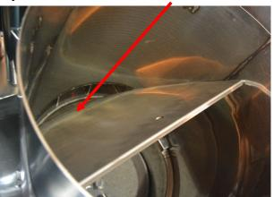
For **ZM-130** – the 'top hat' components shown above rest on the ring, the ring in turns rests upon 3 small pags located around half way up the combustion chamber.
